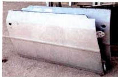
The original passenger-side door showed minimal rust in the front-bottom corner, while the driver-side $50 "swap-meet-find" door returned rust-free. Overall, the L79 looked fine, and now, it's ready to go under the knife. MCR
