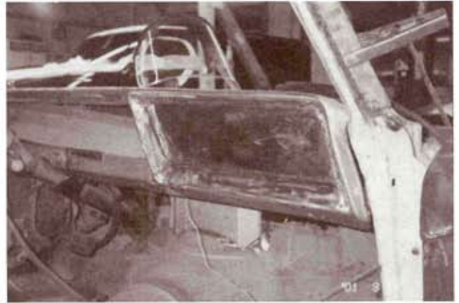
Fabricating dash used parts on another 67 wagon and fabricated the rest.
