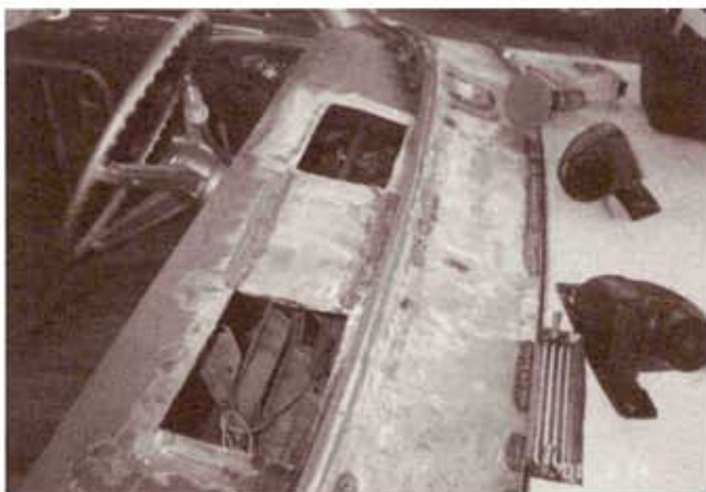
Filled cowl vents and cut out original vent louvers and fabricated and modified the for AC vents new ones.
