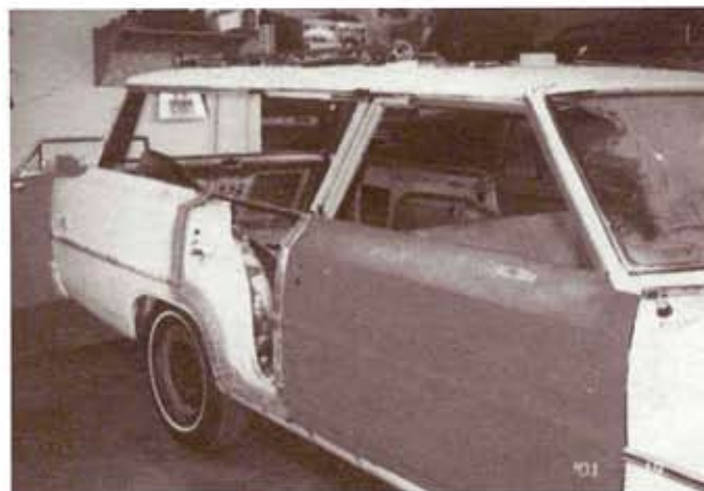
Door hung on and quarter struture framing started. Also laid back of door frame down and eliminated vent glass.
