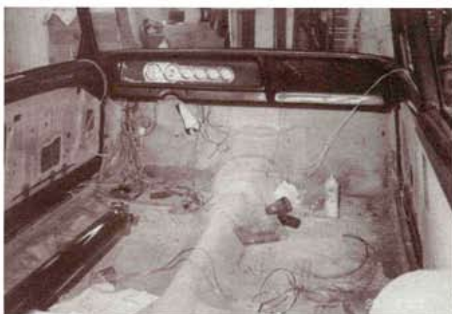
Dash and interior going together. Auto Meter gauges, Billet Speciality gauge cluster, Painless Wiring.
