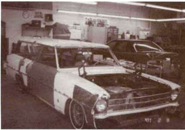
Body with door and post, quarter welded in place sitting in lowered position.
