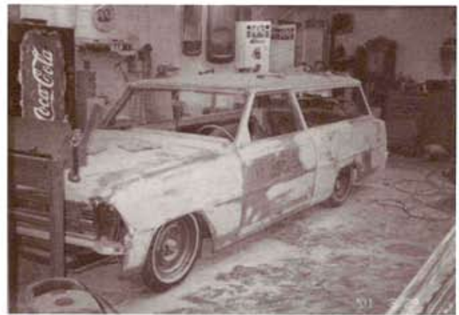
Filler blocked and ready fo primer.
