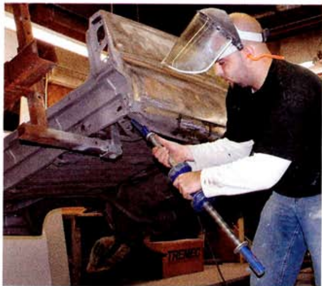
13 Rock worked the metal in the corner using the dent-removing slide hammer, technically called a Morgan Nokker, but more commonly referred to as a slugger. The weight slides down the shaft and strikes the handle, creating a pull on the panel. This process is time-consuming but very effective for removing dents.
