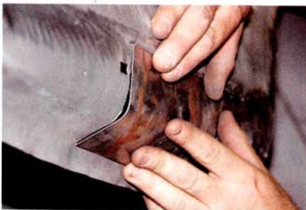
11 Rather than having one big patch, smaller patches were used in order to more accurately follow the factory shape along the bottom of the quarter-panel.
