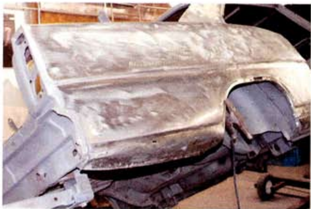
14 After Rock's efforts, the quarter-panel began to take shape, but it still needed repair on the wheel lip.
