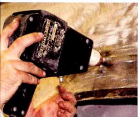
17 An H&S Uni Spotter Delux Stud Welding Gun sent a stud to the quarter at the low point.
