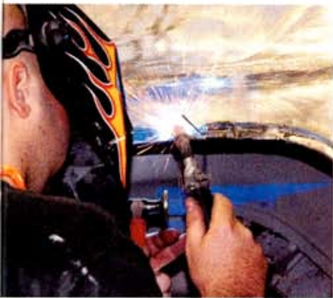
16 Rock welded the metal to the formerly cancerous portion of the wheel lip.
