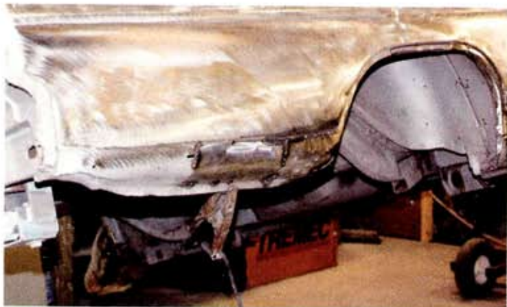
12 At this point, the dent at the rearmost bottom corner must be fixed.
