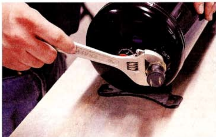
Compressors and tanks are sealed for protection from dust and moisture. A 130-psi pressure switch is installed to the tank to send off/on signals to the compressor when desired pressure is reached.
