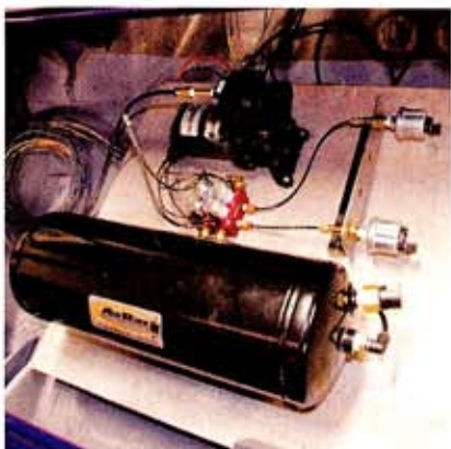
The mounting board slides into the area under the package shelf and will eventually mount the CD changer and other electronic equipment. The board itself will be covered with material matching the rest of the trunk area, completely hidden by a removable panel.
