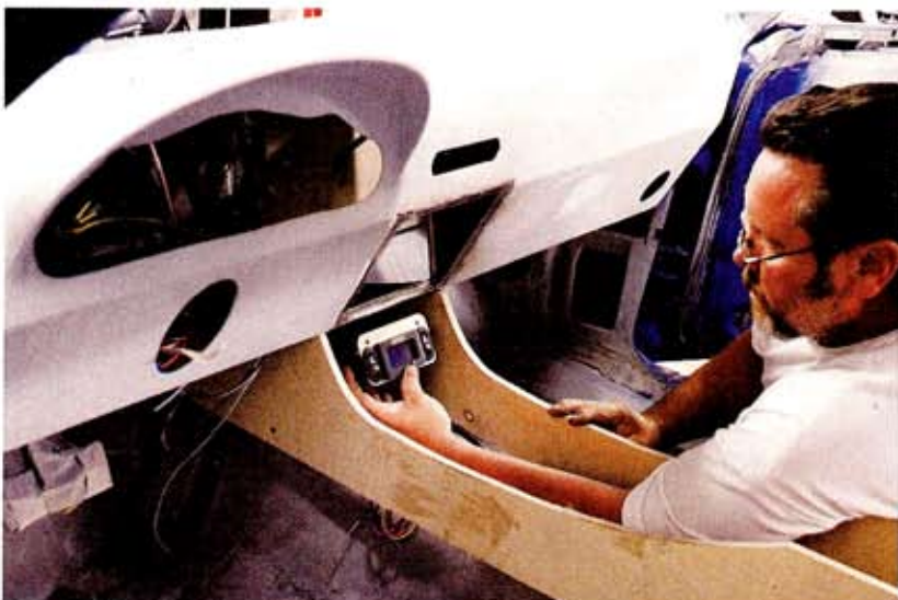
The custom interior includes a shaped console and metal dashboard. Jelinek estimates where the switches will be mounted. We'll show you the final install of Frank Mitello's '69 in the next issue of Camaro Performers.
