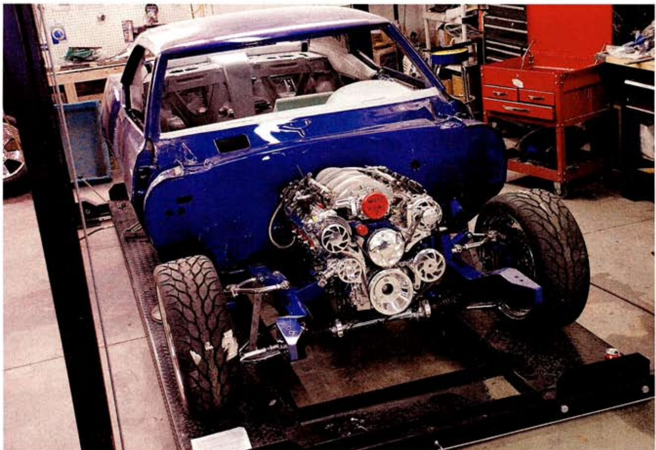
Rt. 66 Motorsports of New Lenox, Illinois, is building this '69 Camaro for Frank Militello. The car features a Chris Alston's Chassisworks front subframe, smoothed firewall, an LS2, and a custom interior.
