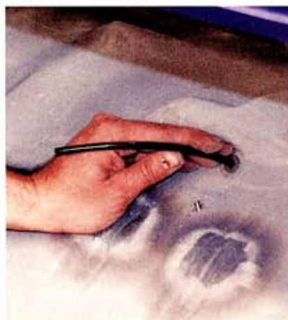
The hole will eventually be fitted with a grommet for a nice tight seal.
