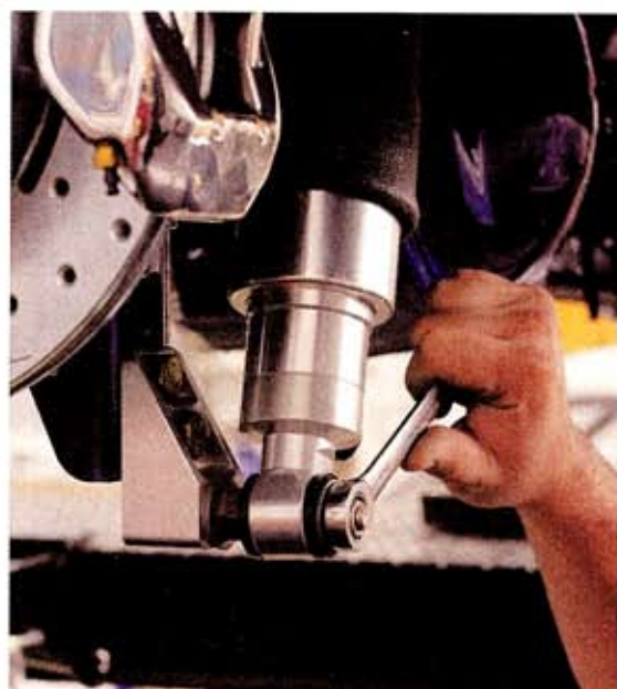
The ShockWave 7000 is specifically designed for the lightweight Camaro. The Firestone sleeve-style air spring offers more travel and a softer spring rate, shown effective for the solid axle rear suspension.
