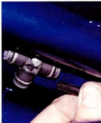
Referred to as a two-way system, one switch will control pressure in the front Shockwaves, and one switch will control pressure to the rears. Matt attaches the airline to the supplied T-fitting. Pressure is then routed to both the right and left sides.
