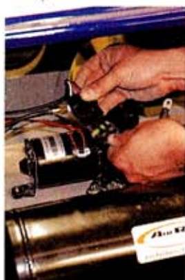
Wires from the solenoid are simple weatherpack-style plug-ins. Now the airines from the ShockWaves can be installed.
