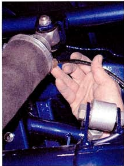
The airlines are also attached to the driver's side ShockWave 7000. With the lines tucked up along the AirBAR, they virtually disappear.
