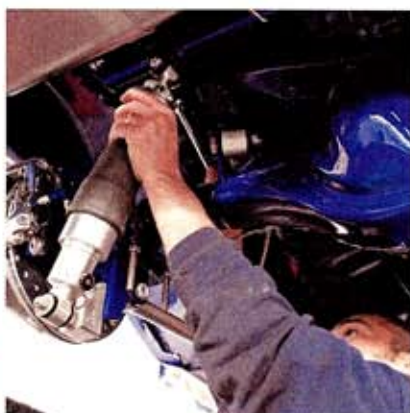
Matt Duque of Rt. 66 Motorsports knows these systems well. Fittings are tightened with extra care to avoid scratching the GM Impulse Blue paint.
