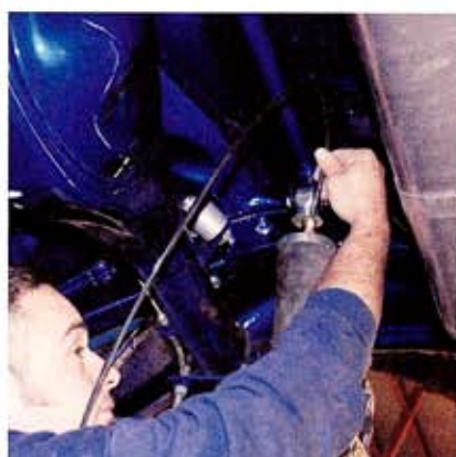
Matt attaches the supplied 1/4-inch line to the ShockWave. The 16-position shock adjuster allows the driver to dial in the exact level of ride stiffness and performance.
