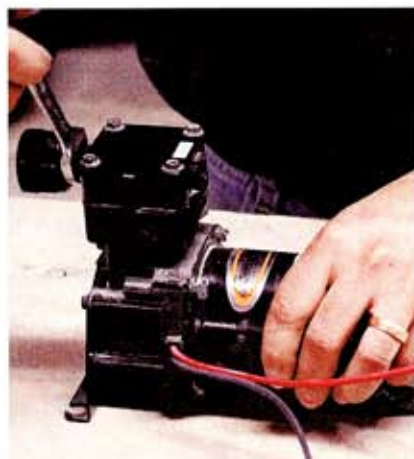
The compressor is fitted with the air screen at the inlet.
