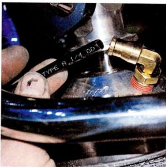
The air line is now able to be installed into the fitting on the ShockWave.
