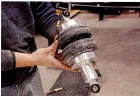
Ready to be installed, these Air Ride Technologies ShockWaves are built to last. The design has been around a long time on those 18-wheelers, so this lightweight Camaro is receiving proven technology.
