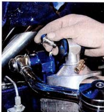
The top-mount fastener is inserted and tightened.
