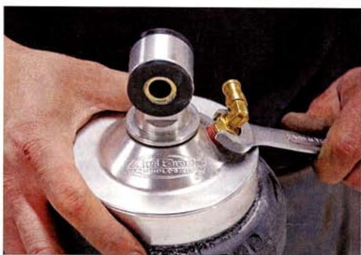
The air line elbow fitting is installed into the top of the ShockWave.
