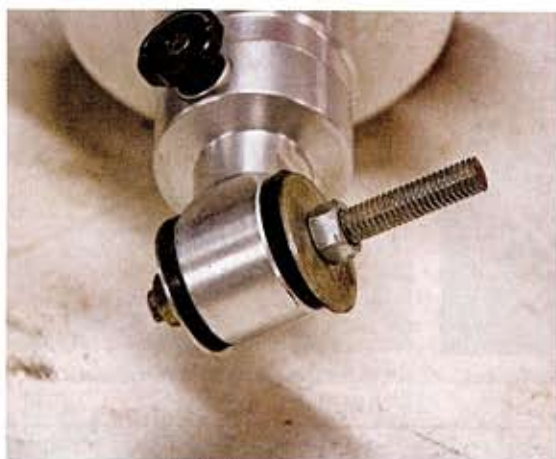
In order to install the bushings top and bottom, take two large washers, the longer bolt and nut, and press the bushings in place.
