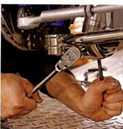
With the fastener inserted, the ShockWave is tightened at the bottom mount.
