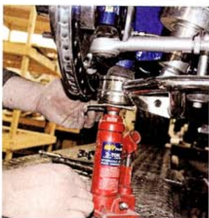
A small hydraulic jack helps align the hole for the bottom shock mount.
