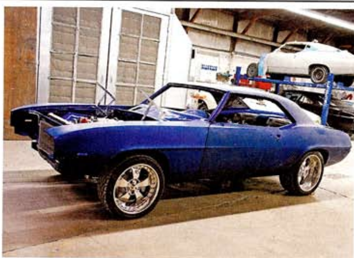
With the complete Air Ride Technologies suspension installed, the ShockWaves are filled to the maximum ride height. The car still needs front metal and glass, and the interior is still missing, but the installation will only lower the car slightly.
